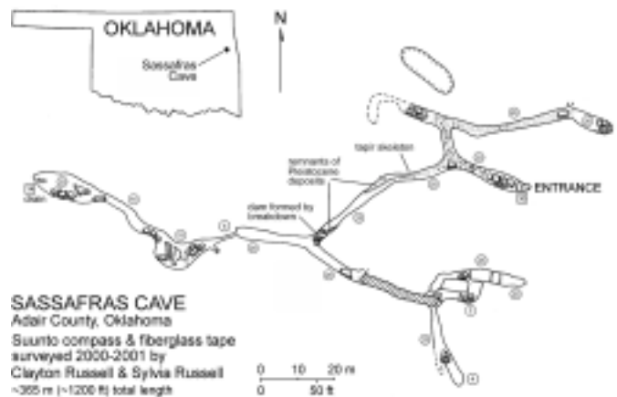
Figure 1. Location map and plan view of Sassafras Cave, showing discovery site of tapir skeleton in a Pleistocene terrace. NSS standard map symbols follow Hedges et al. (1979). Ceiling heights (encircled numbers) are given in feet.
