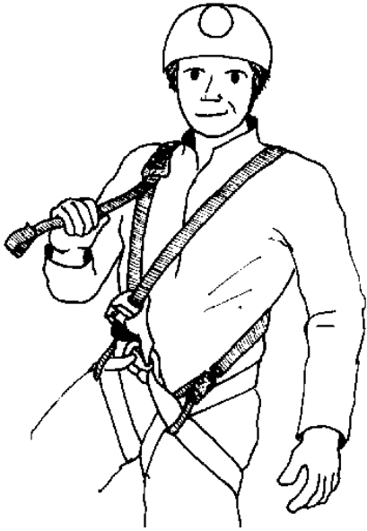
A chest ascender attached to the seat harness is held up with a chest harness.
